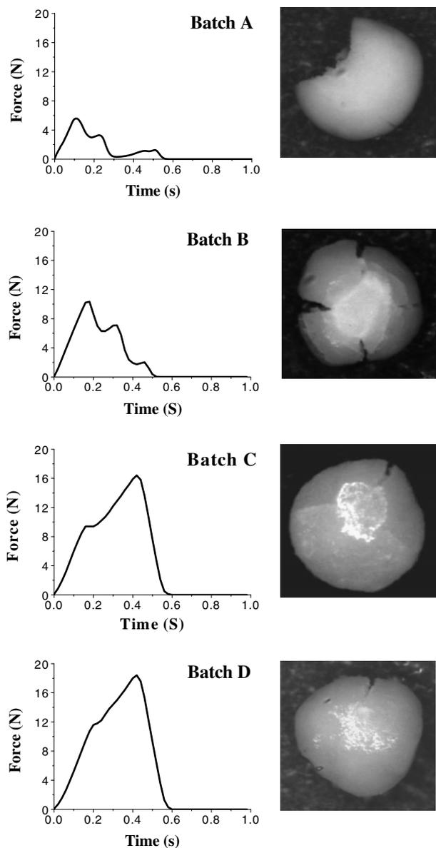
Fig. 2. Examples of crushing strength plots and the corresponding images of the crushed pellets for the four batches of pellets. Images were taken after the first peak or notch.
