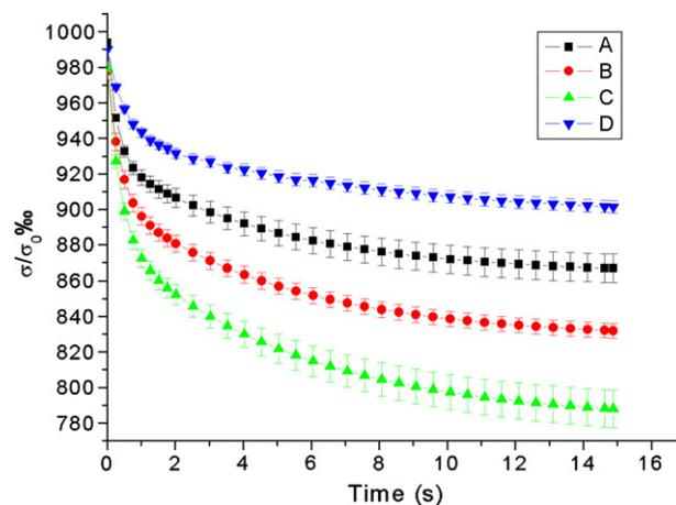
Fig. 4. Stress relaxation curves of the four batches of pellets.
