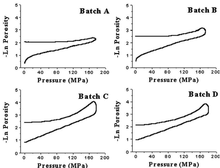
Fig. 5. Heckel plots of the four batches of pellets.
