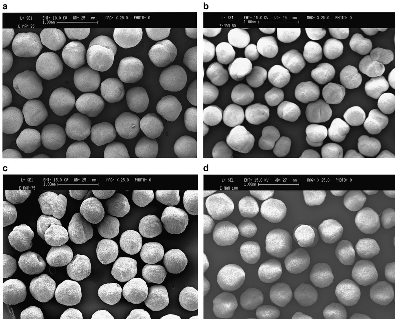
Fig. 1. (a–d) SEM images of the 600–710  $\mu\text{m}$  batches of pellets.
